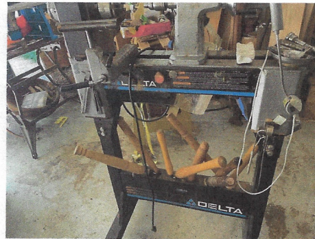
Delta lathe. 115V, reversible, variable speed motor
