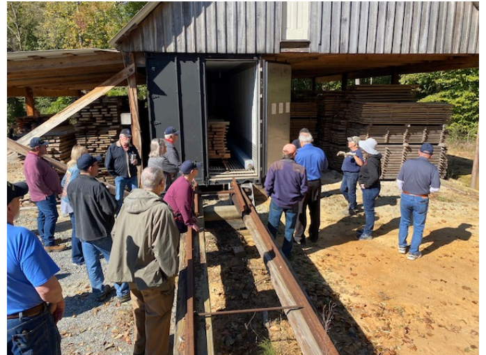
Leigh opened the door to the converted trailer/dryer oven to show how cut lumber was stacked for the 3-5 day drying process.
