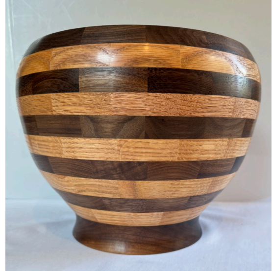
Segmented bowl with 10 rings of oak and walnut. Walnut base. Finish is Danish Oil (Tried and True), then buffed. Top coat is carnauba wax topped with Renaissance Wax.
