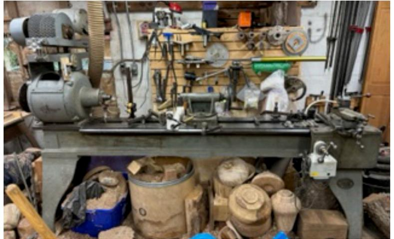
Yates American lathe. 16" swing inboard and 5-6' outboard. Between head and tail stock is almost 6 feet. Plenty of room for most architectural spindle turning and/or large bowls/platters.
