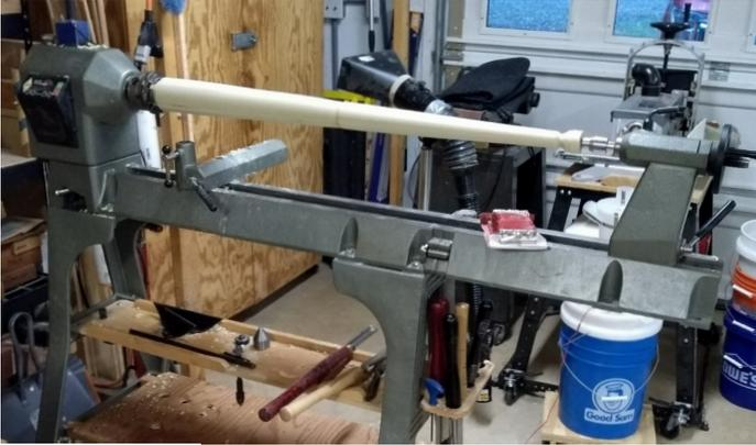
My steady rest is not large enough for the Nova lathe and I had to raise it up by using a piece of plywood as a riser block. It still couldn't support the thinner end. At that point, I could sand the cones using this configuration but not turn them. So, in conclusion, the first one is not done as well as I would like. The second one came out looking much better.
