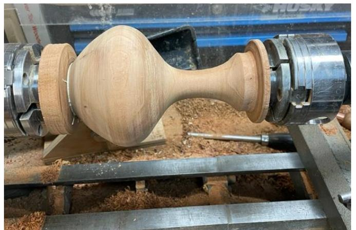
This is one of my hollow-from-the-bottom challenge pieces getting the bottom plug installed and before completing the top.
