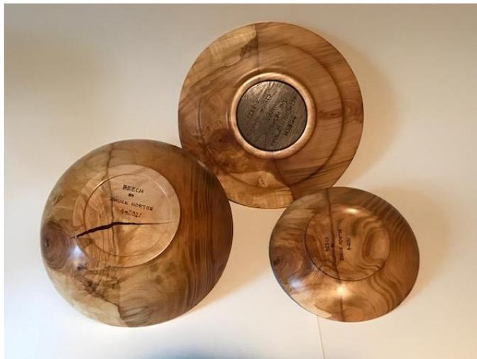
The platter has a walnut insert in the base because it warped so much in drying that the bottom was quite thin. It also has a heart insert in the top side to conceal tearout. The crack in the large bowl was filled with dyed polyester resin.
