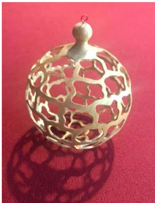
The above are photos of the two pieces Dan worked on in the demo. The spherical one is the one he finished on the lathe and began piercing. The other is the one he began turning, glued up, and set aside. Since there was some extra wood in this one, he elected to make it into somewhat of a teardrop shape. Note that he stopped piercing before reaching the top since the inside is still spherical, and the wall at the top began to get too thick to pierce.
