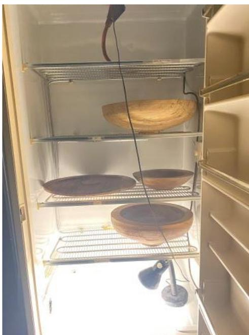
The bowl blank started out at 57% + moisture on February 18, 2021 in her homemade kiln from an old freezer. It has vents in the top and bottom with a fan for circulation. On March 18, 2021 the rough turning was about 34% moisture content. It was finished turned on May 1st at 10% moisture.
