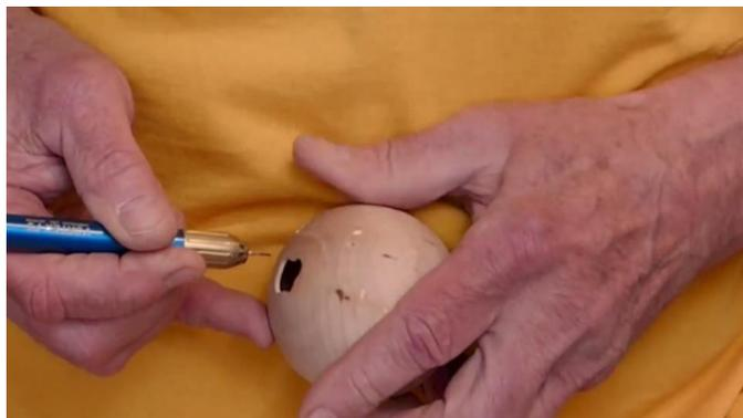
Use a high-speed dental tool for best results. You can also use a Dremel, but the cutter is larger, the speed is slower, and it tends to vibrate. Start piercing and clean up any burn marks with a light touch.
