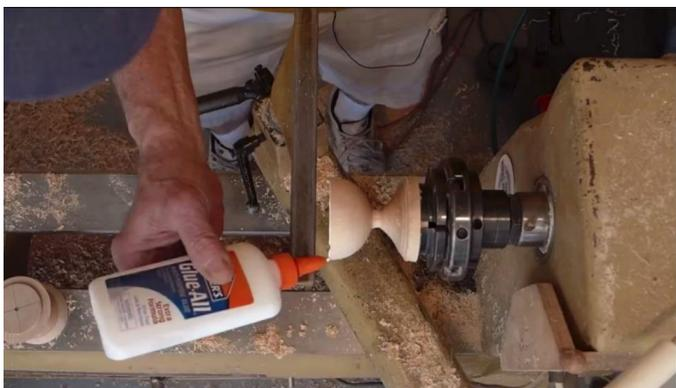
This is a complete hemisphere, ready for gluing to another hemisphere. Wall thickness is 1/16" ±.
