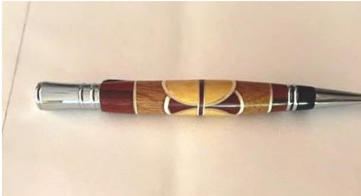
The final design uses a mortiser with a 1/4" bit to create diamonds in the blank. The opening is then filled with a 1/4" by 1/4" piece of wood or other contrasting material. The remainder of the blank is created by cutting small pieces of wood at a 45-degree angle and then gluing them together as shown.
