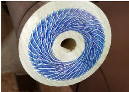
Here I used the same mini-tool set it at a slight angle, about one o'clock position, then moved the tool to the left while I continued to rotate the tool to about a two o'clock position near the edge. Again, it was colored and highlighted for a better picture.
