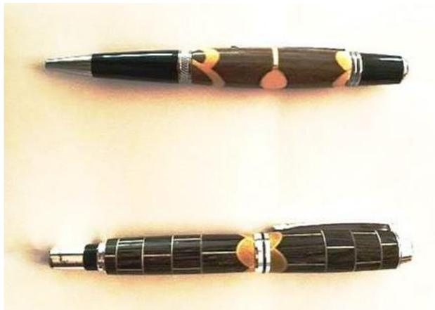
Another interesting technique is the use of medallions as shown below. These appear as circles on the blank. These are created at the drill press using a hole saw, with a jig and stop to ensure consistent locations for the medallions. Only a small piece of the hole saw cuts through the blank. After cutting each medallion, a replacement piece is glued in its place. The same material, contrasting material, or a "sandwich" of materials can be used, similar to doing scallops.
