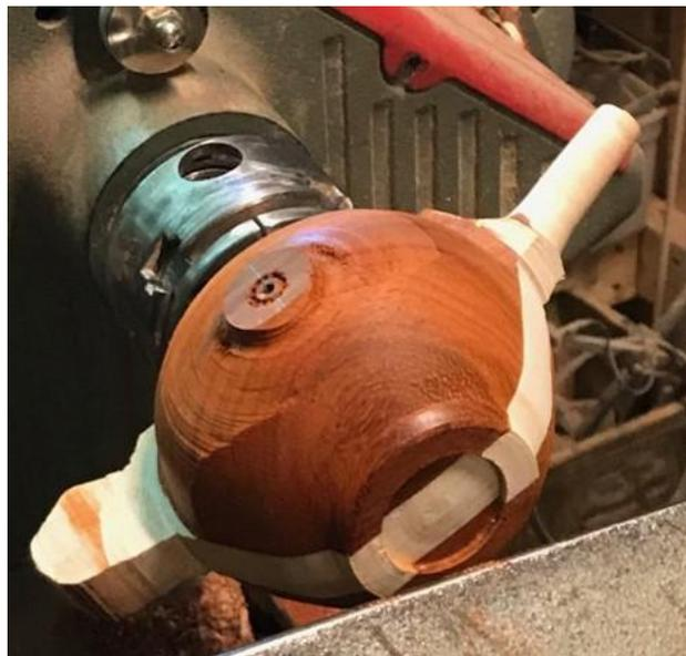
If necessary, you can remount the piece between centers and adjust the sides being very careful not to cut off any of the bottom recess. After doing any necessary tweaking, use the bottom tenon for mounting in a four jaw chuck to shape the top and hollow the piece.
