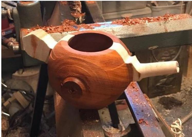
After completing turning on the lathe, I use a marker to finalize the basic shape of the handle. I also use a circle template to locate and define an outline of the feet on the bottom rim around the recess that I turned for chucking.
