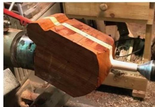
After turning the spout, I took the piece back to the bandsaw and trimmed off some of the excess on both sides of the handle.
