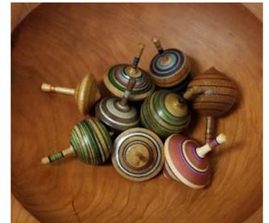
To do the touch up and to mark the lines, he used a small skew. Next, he turned the lathe down to 130 rpm and used a green marker to paint over the engraved markings. Lines in black marker were used to border both sides of the green, engraved space.
