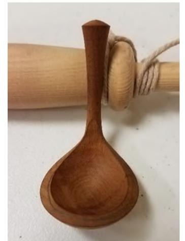
Turning a simple two axis cherry spoon. I use a NOVA DVR, and a NOVA G3 chuck with a Vermec/Vicmarc eccentric adaptor. Tools used are 10mm and 12 mm shallow gouges, a 5mm bedan, a shear scraper, and a 1/16" parting tool.
