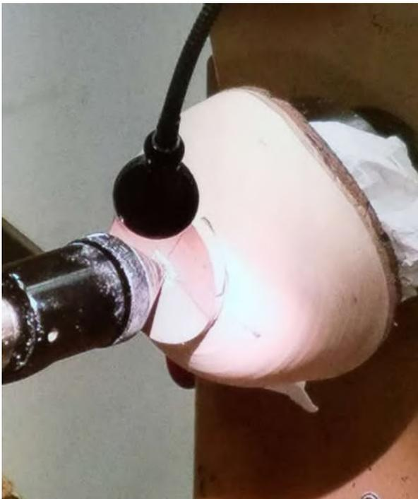
*THE INSIDE IS FINISHED AND THE PIECE IS REVERSED ON THE CHUCK WITH A BUFFER OF CLOTH COVERING THE CHUCK. THE TENON IS REMOVED TO FORM A SUITABLE FOOT*
