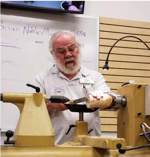
*NOTE THAT THE WORK PIECE IS MOUNTED WITH GRAIN PARALLEL TO THE LATHE BED*
