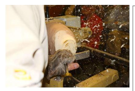
Use the horsepower that came with the lathe. Don't just nibble away at the wood. The objective in roughing is to get it into the bag for drying.
