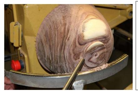
On scroll chucks use compression fits vs expansion fits to attach wood to the blanks. It is much stronger to attach blanks to the chuck in the compression mode for most people.
