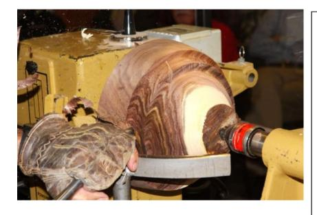
Turn the blank by using a cut that is into the side grain. Don't try to cut the end grain.
