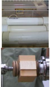
ring for the rotating cylinder. Mirrors are first surface and you need 3 cut (get a good glass cutter with oil). Tape the mirrors together (silver up), peel off blue cover, fold up and duct tape the whole thing (no finger prints on mirrors). Silicone drops at the end to hold mirrors inside
