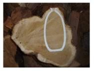
2. **Centering the grain at the bottom of the bowl.** Keep in mind where the pith is, if you want the grain concentrically centered at the
