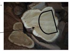
**3. Aligning the blank** With a blank like this one, I insert a spur drive in my chuck—I'm lazy—in order to reach into the center recess. I pin the blank between the spur and the tailstock, rotate it and adjust the tailstock until the high points and the dips line up reasonably well. I put my hand on the tool rest and use my finger to align the tips and dips.
