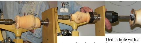
Forstner bit, slow down the speed and clear out the chips often. Work from the top down into the form (you can't go back as the wall will be too thin and might warp. Use all your hollowing tools (straight, angle, swan neck, arm holders, laser, etc). Cut at center line or just above to leave an escape path for possible catches. Clean up the inside with light strokes using a scraper. Jam chuck it to finish the bottom. Concave it a bit, cut off and sand. **[Continued on page 2]**
