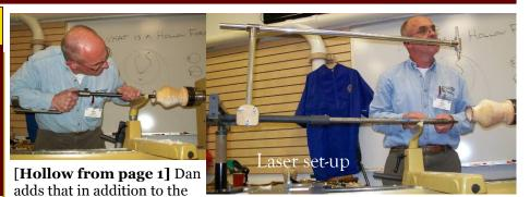
scraper used with the Sorby swan neck tool he used, it is also supplied with a 3/16" tool steel cutter , which is much less aggressive than the tear drop scraper, and should be used for roughing. The tear drop scraper is used for light, finishing cuts.
