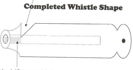
3/8" dowel sanded flat on top and glued in place. This channels the air past the "V" cut causing the whistling sound. Before gluing, test whistle for correct dowel placement.
