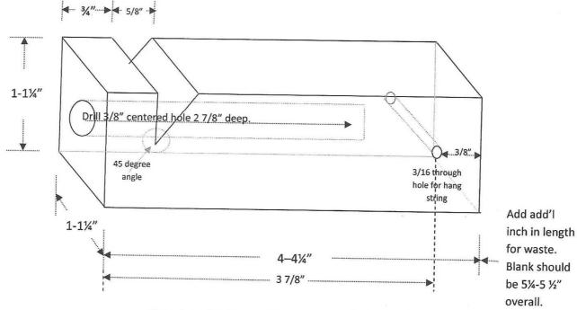
Complete all drilling and band saw cuts before turning.
