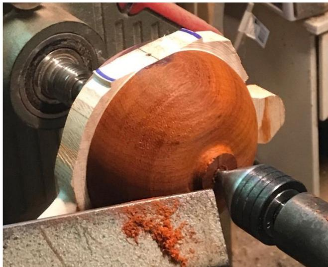
Despite creating a reference for the bottom, I ended up cutting in to the area that I had planned on leaving for the bottom recess. The reference simply kept me from going even farther and ruining the blank. After turning both sides, I remounted the piece using a worm screw and adjusted the bottom, turned a recess, and shaped the bottom up to my side mounting points.
