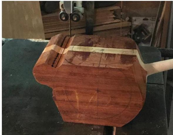
This next step is not necessary but I find it useful to create a reference for maintaining an area for the bottom recess while rounding the sides. I drill a hole in the top and mount the piece in the four jaw chuck using a worm screw. I then partially round the bottom to locate the outside diameter of the mounting recess.
