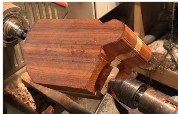
After turning the tenon, I flip the piece around and mount it in a four jaw chuck and then drill a hole through the spout to a depth where it will later be hollowed using a Jacob's chuck. I then turn the spout round.
