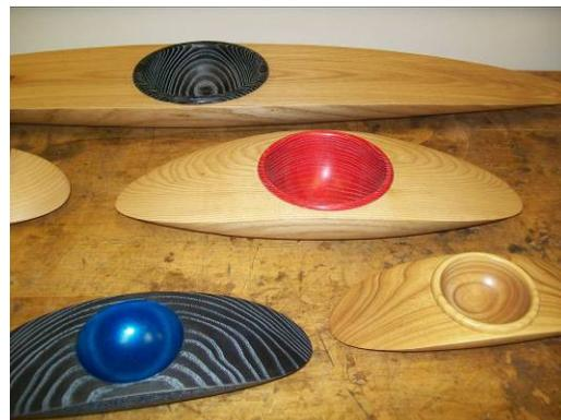
Brian turns a cylinder first then makes little "V" cuts to mark the center (pencil marks get turned away). He turns the curvature on one side out from the center and the other side is a mirror image; he measures to make sure so it's balanced. Brian likes the football shape and turns the tips to 3/4 thickness at the edge. He sands #150 on the lathe and the final 2 grits are sanded with the grain and off the lathe.
